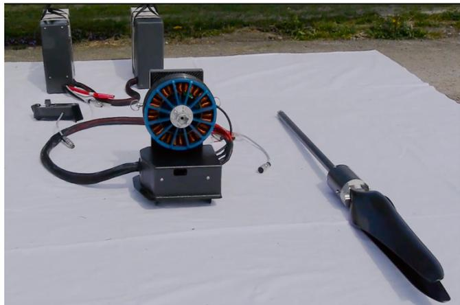
The electric launch aid has only a few minutes endurance, which is enough to reach the first thermal or ridge ; it replaces aero-towing, or winch launch, which are not easy to operate, or foot launch where safety margins are not as high as for paraglider or hang glider pilots.
